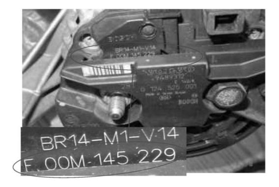
The old regulator (P/N 9459741) can be identified by the Suppler P/N FOOM 145 229 (See picture) And the new regulator (P/N 8637851) by the Supplier P/N FOOM 145 279
